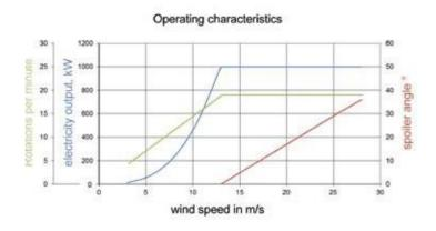
The *operating characteristics* graph demonstrates how the spoilers control rpm and energy production under high winds.
